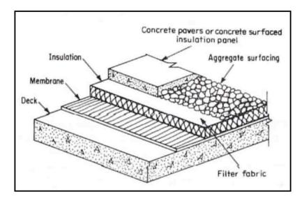
Above is a detailed drawing of the cross section of an IRMA system. Notice the attachment of the roof system directly to the deck followed by the insulation.
